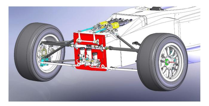
The front nosebox will be installed 5mm forward compared to the 2017 position, the bolts and the front damper cover will be provided in the update kit.
