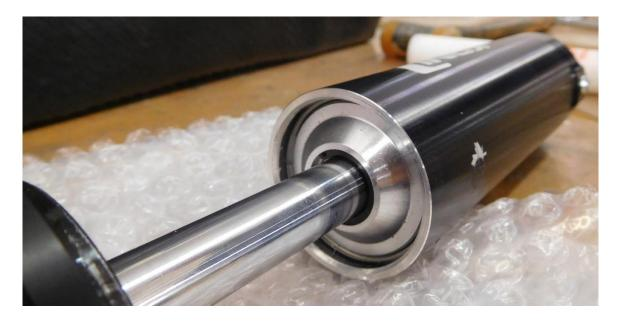
Once cleaned, with the help of a plastic mallet fit back the platform
