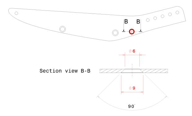
Please note that also the countersink on the flap could need to be adjusted accordingly.
