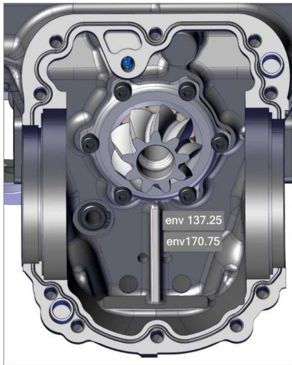
Measure the highest distance between the external races of the bearings assembled on the differential case and note it: this is dimension "Y"
