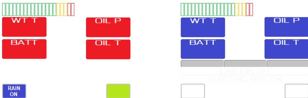
All the value boxes turn red when the value is over the maximum (alarm values are set by engine control), and blue when the value is below the minimum, all the alarm messages can be skipped pushing AKN button.
