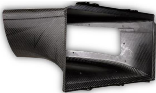
Picture 1: Lh sidepod before trimming
