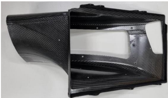
Picture 2: Lh sidepod after trimming
