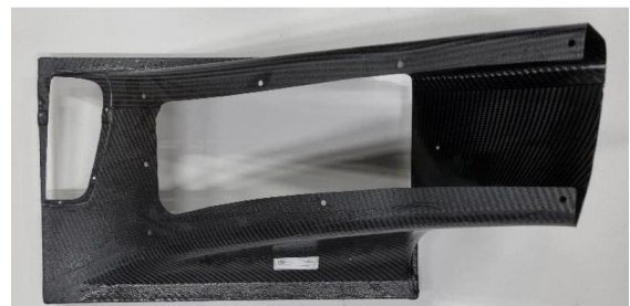
Picture 2: Lh sidepod after trimming
